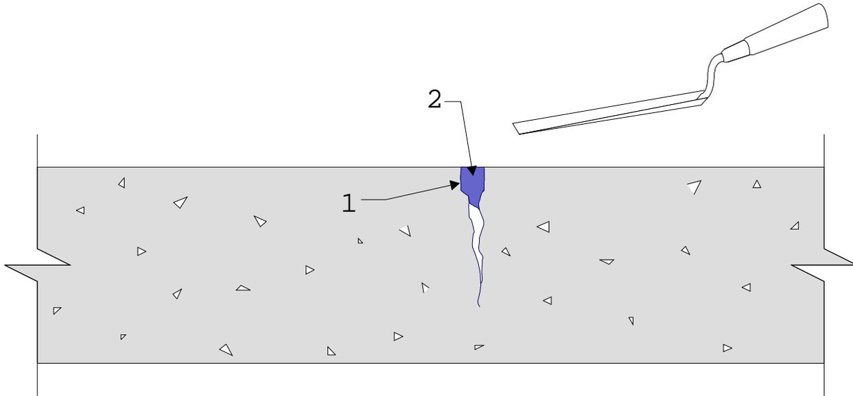
1. Prime prepared substrate with neat Sikadur 21 Lo-Mod LV epoxy resin adhesive binder.
