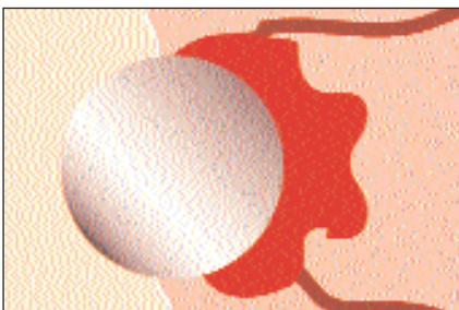
Volume Expansion of Rust Causes Cracking and Spalling
