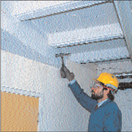
Hammer Testing for Soundness
