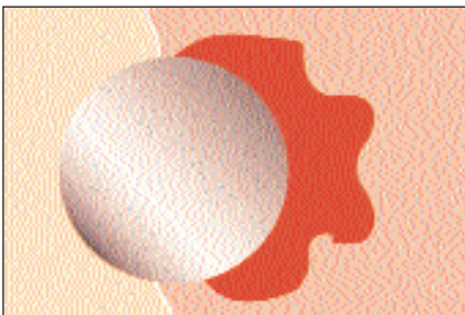
pH at Steel Drops Below 9.5, Corrosion Begins
