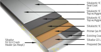
Seal Coat Sikalastic 1C Top w/Aggregate Sikalastic 1C Top w/Aggregate (as Reqd.) Sikalastic 1C Base
