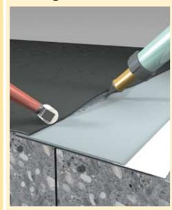
Weld (with hot-air gun or with welding machine) the PVC side of the Sika® Dilatec® R-Edge with any PVC-type waterproofing membrane or building com-
