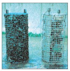
Sikadur Combiflex After 12 Month Immersion in Raw Sewage and Potable Water
