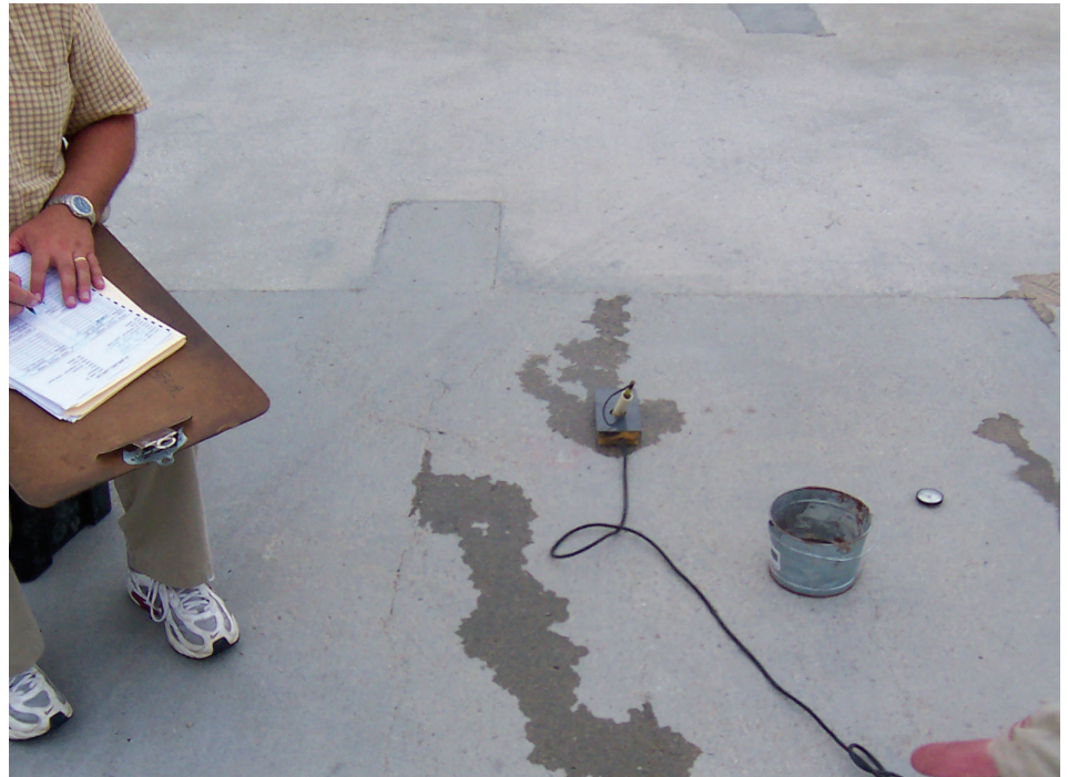
Half-cell corrosion potential testing
