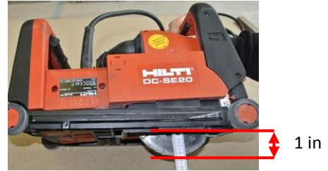
Depth of incision: The joint cutter must be adjusted to a depth of 1 in.
