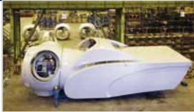
Giant of the Sea A 5-MW megawatt wind turbine by Repower Systems being built for the Beatrice project. Its place of operation is the open sea in the Moray Firth, East Scotland.
