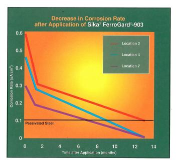
before and after application of the FerroGard 903 to determine its effectiveness. A testing lab was hired to measure the corrosion rate in different areas of the building over time. The graph shows the measurements in an area that was treated only with the corrosion inhibitor, and indicates that the corrosion rate decreased (tested in according with ASTM G 3)
