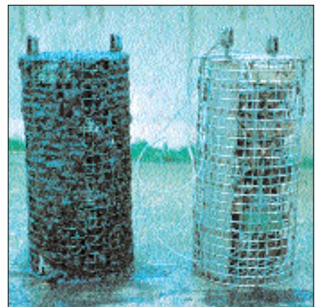
Sikadur Combiflex After 12 Month Immersion in Raw Sewage and Potable Water
