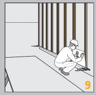
Place the cladding panel in the required position first, without the panel touching the fixing tape. Then, press it firmly until it touches the SikaTack® Panel Tape.
