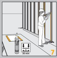
Apply SikaTack® Panel-50 in a triangular bead by using a triangular nozzle (width 8 mm, height 10 mm) with at least 5 mm gap to the fixing tape and to the side of the batten.
