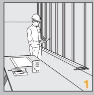
A well prepared working place is important for working with adhesives. Mark precisely where the first panel must be bonded on the substructure, or use a reference fixed on the substructure. Make notes for your record with all relevant informations.
