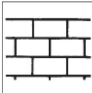
**Description:** 4" x 7 3/4" bricks with 1/2" mortar joints arranged in a running bond pattern.
