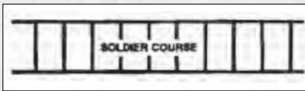
**Description:** 3 5/8" x 7 3/4" bricks with 1/2" mortar joints arranged in single file for borders.
