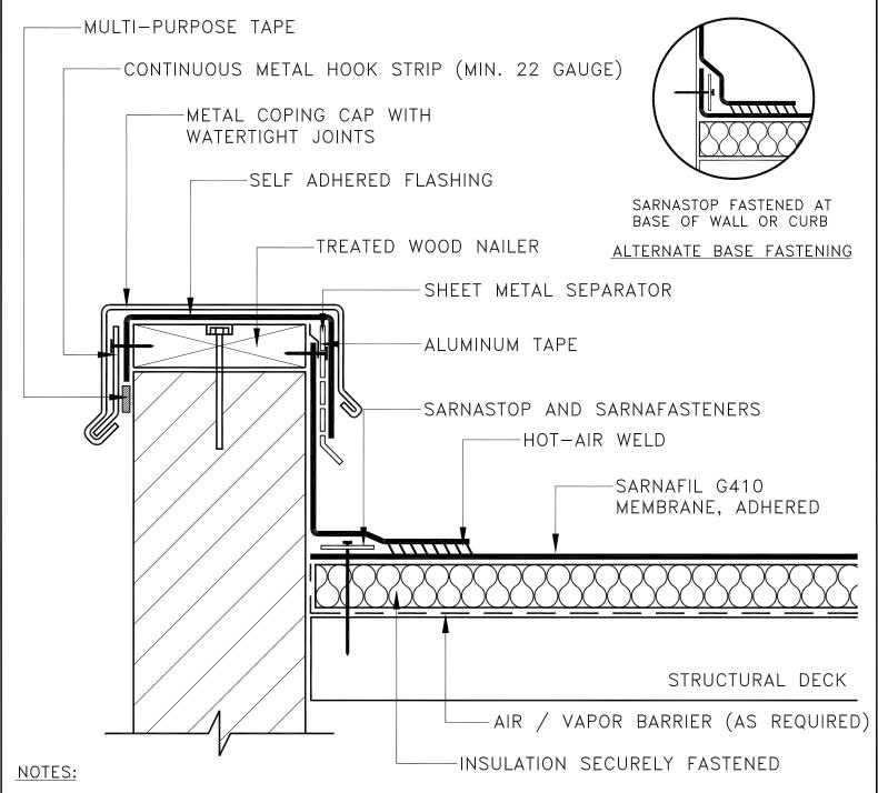
1) NAILERS SHALL BE SECURELY ANCHORED TO THE DECK TO RESIST A MINIMUM FORCE OF 300 POUNDS PER LINEAR FOOT. REFER TO FACTORY MUTUAL DATA SHEET 1-49.
