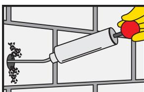
The drill hole must be cleaned with a blow pump or by compressed air, starting from the bottom of the hole (at least 2x). Important: use oil-free compressors.
