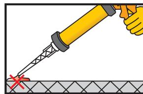
Pump approx. twice until both parts come out uniformly. Do not use this material. Release the gun pressure and clean the cartridge opening with a cloth.
