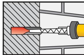
Inject the adhesive into the hole, starting from the bottom, while slowly drawing back the static mixer. In any case avoid entrapping air. For deep holes extension tubing can be used.
