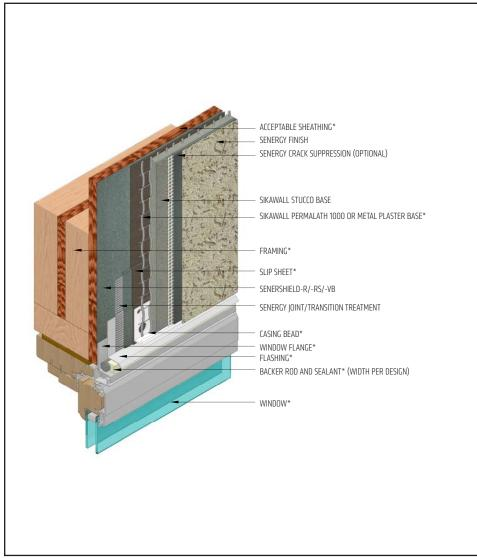
Prior to window and lath installation, ensure water-resistive barrier is properly applied into the rough openings in accordance with Senergy application guidelines and code requirements. Reference Senergy Senershield published typical details for further information.
