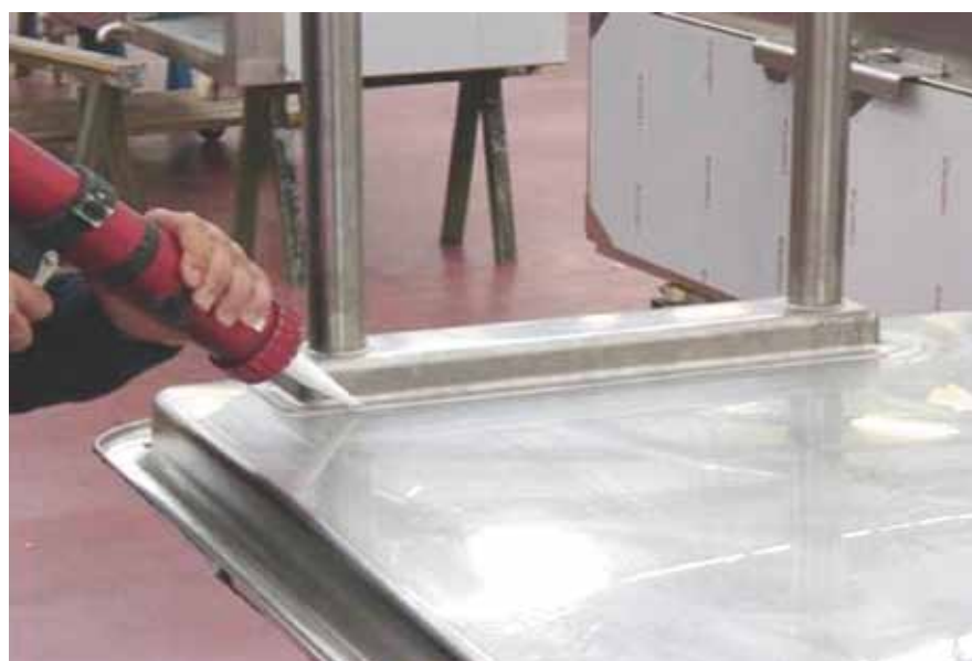
Fig. 87 Metal table legs are bonded and sealed to a metal table-top using Sikaflex®-292
