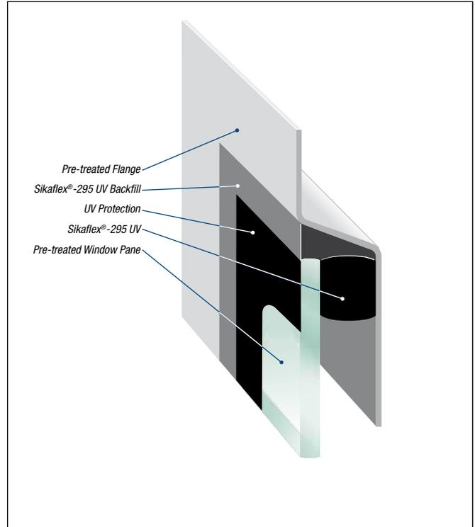
Fig. 124 Typical construction of a window with outer UV protection
