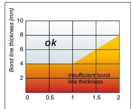
Fig. 127 The bond line thickness to largest pane dimension (m)
