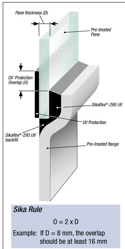
Fig. 125 Minimum Recommendations for UV Bond Line Protection
