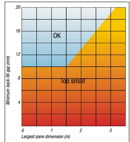
Fig. 126 Back-fill gap to window size ratio
