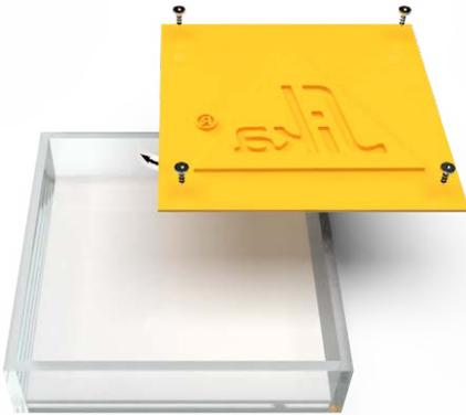
**1** Fasten formliner to form using mechanical fasteners, adhesive, or tapes. Ensure the correct side of the liner is facing the formwork (Sika formliners have a tag indicating the formwork side.)
