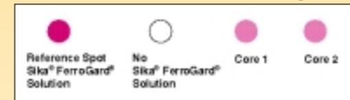
Sample of color indicator using on-site gas chromatography to detect presence of Sika® FerroGard® 903 in concrete cores.
