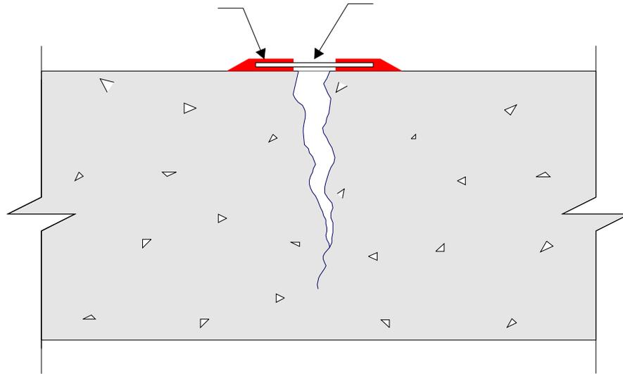
1. Wipe Hypalon sheeting with Combiflex Activator a minimum of 1 hour and a maximum of 8 hours before installation.
