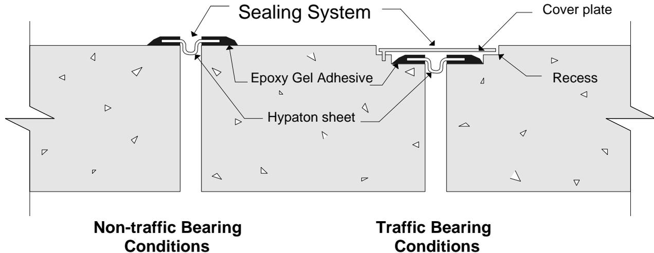
1. Wipe Hypalon sheeting with Combiflex Activator a minimum of 1 hour and a maximum of 8 hours before installation.
