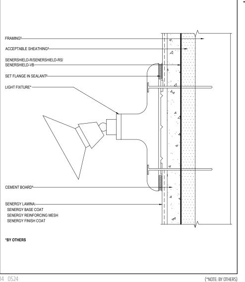
• Ensure all penetrations into the system are properly sealed.
