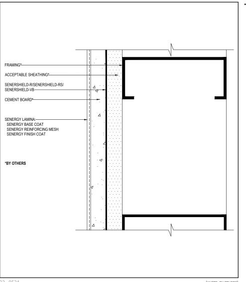
Install Senershield per published details and product data sheet prior to the installation of windows and SikaWall Drainage Mat.
