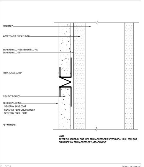
Locate control joints approximately every 600 ft.2 (56 m<sup>2</sup>) of wall surface area with maximum uncontrolled length or width of 24 lin. ft. (7 m) and a maximum uncontrolled length-to-width ratio of 21/2:1.
