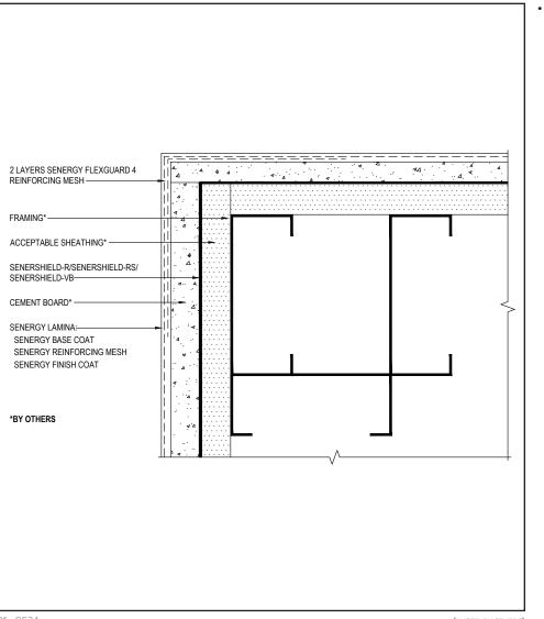
Ensure Flexguard 4 Reinforcing Mesh is lapped a minimum of 8" (203 mm) around corner on both sides.
