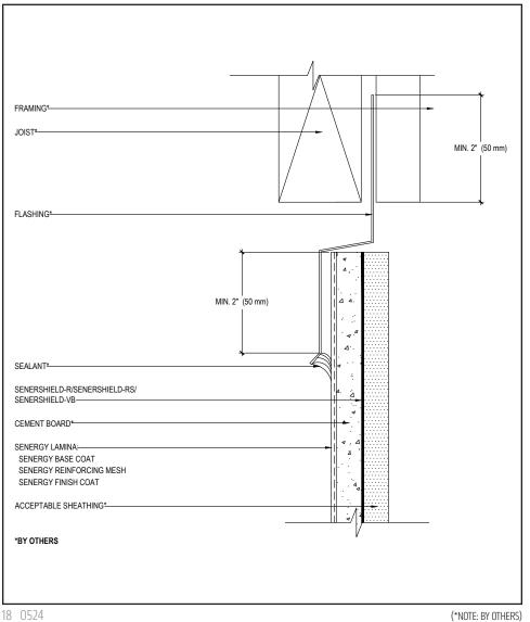
Ensure that metal flashing extends onto the system a minimum of 2" (50 mm) down the face of CBS 1000 system.
