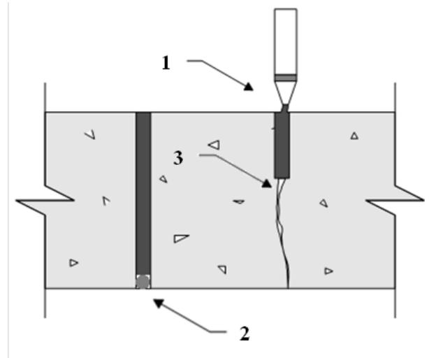
1. Pour Sikadur®-58 CJR into prepared joint and allow to overflow
