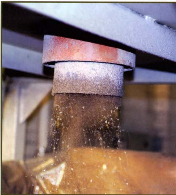
Figure 7 – PVC membrane being ground for recycling.
