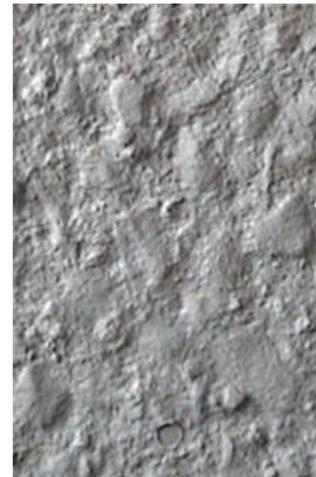
CSP-7, Heavy Abrasive Blast
