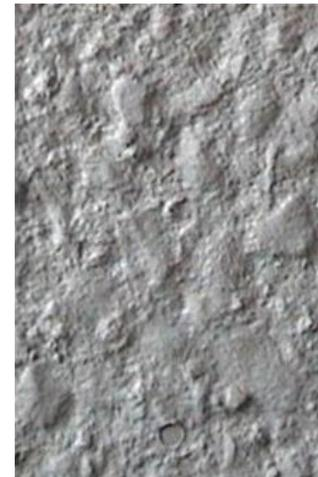
CSP-7, Heavy Abrasive Blast
