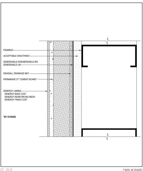
• Install PermaBase CI composite cement board panel over Senergy air/water-resistive barrier and SikaWall Drainage Mat per manufacturers' recommendations, applicable building code and project requirements.
