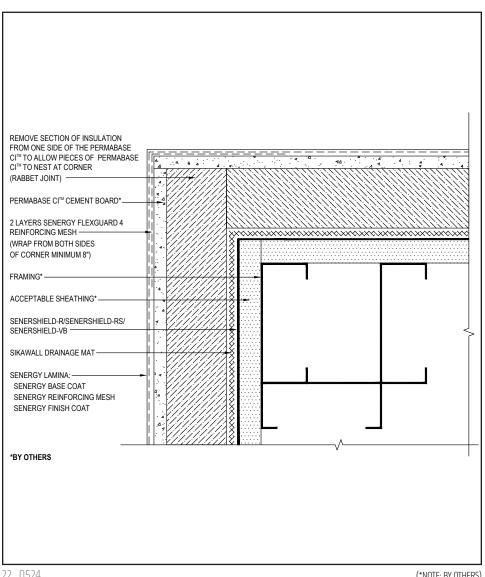
• Ensure Flexguard 4 Reinforcing Mesh is lapped a minimum of 8" (203 mm) around corner on both
