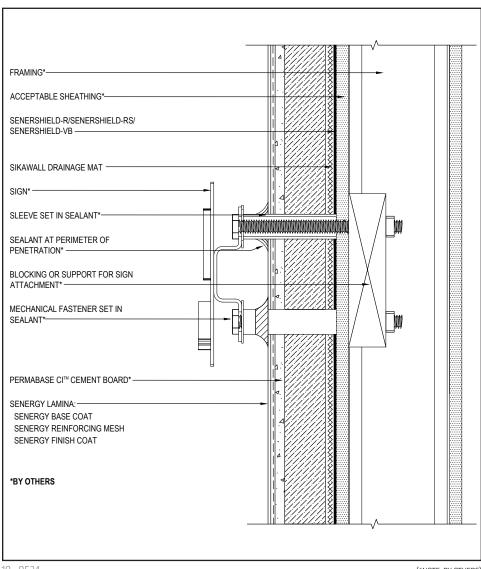
Ensure all fastener penetrations through the system are properly sealed.
