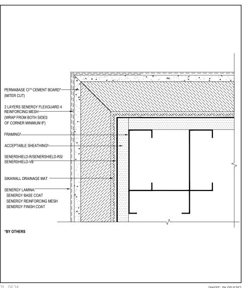
Ensure Flexguard 4 Reinforcing Mesh is lapped a minimum of 8" (203 mm) around corner on both sides
