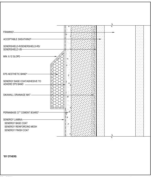
On horizontal projections greater than 1" (25mm) maintain a minimum 6:12 slope. For sloped surfaces over 24" (340mm), a roofing system or a metal cap flashing is required.
