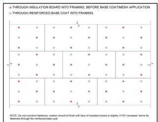
a. Spot all exposed fasteners (fasteners on outside of reinforced base coat) with Senergy base coat prior to application of final skim coat layer of base coat. Multiple coats of base coat may be required to achieve a flat surface.
