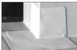
11. After welds are thoroughly cooled, check all welds with a rounded screwdriver blade. Re-weld any inconsistencies.
