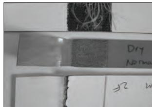
Typical seam break of good welds.
