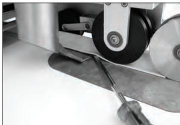
Fig. 1.8 Lifting the rib to insert the welding machine nozzle
