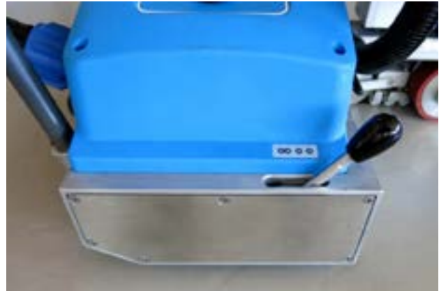
Neutral gear for easy movement on the roof.
