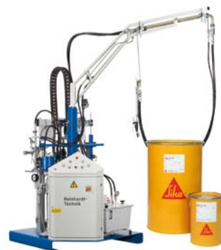
top: Application machine for 2-part sealants out of drums and pails (factory application)
