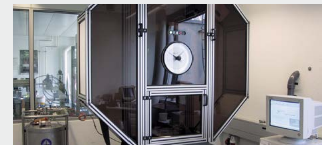
Impact test machine with pendulum (ISO 11343) for velocities of 1 m/s to 5 m/s at temperatures from -50 to 80 °C (-58 - 176 °F). As glass deforms with a max. speed of 4 m/s, this is the optimal range for simulating bomb blast tests.
