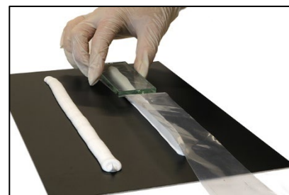
Figure 13 Press the bead to half the height
