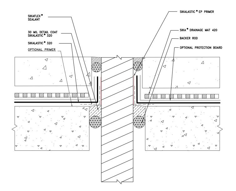
NOTES: REFER TO SYSTEM GUIDE FOR PRIMING, SIKALASTIC 320 THICKNESS, PROTECTION BOARD, AND DRAINAGE MAT REQUIREMENTS
