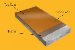
Sikafloor MultiDur combines performance and versatility for use in high demand commercial and industrial settings. MultiDur is an versatile coating system and can be designed to tolerate aggressive surface conditions such as heavy traffic, large equipment, abrasion and harsh chemicals.
