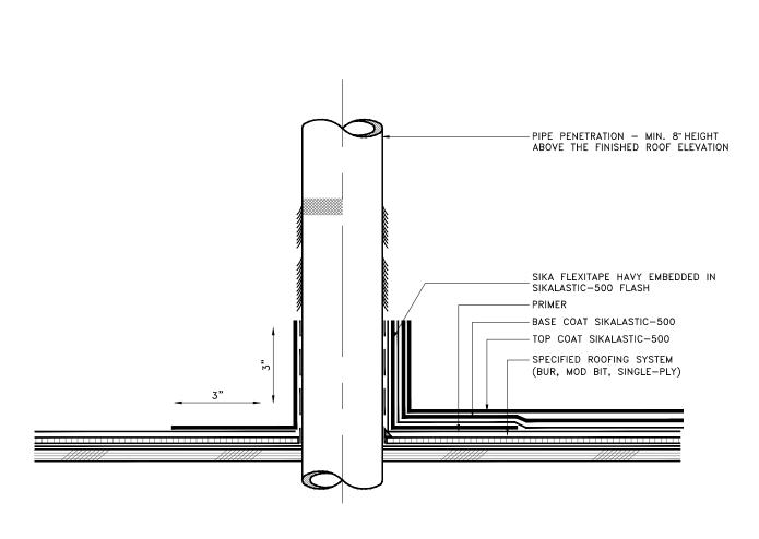
NOTE: ADD SIKALASTIC FLEXITAPE HEAVY 6" ON METAL EDGE FLASHINGS, AND ON ALL PENETRATIONS.
