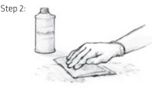
Clean contaminated surface with approved solvent such as acetone, MEK or Xylene.
