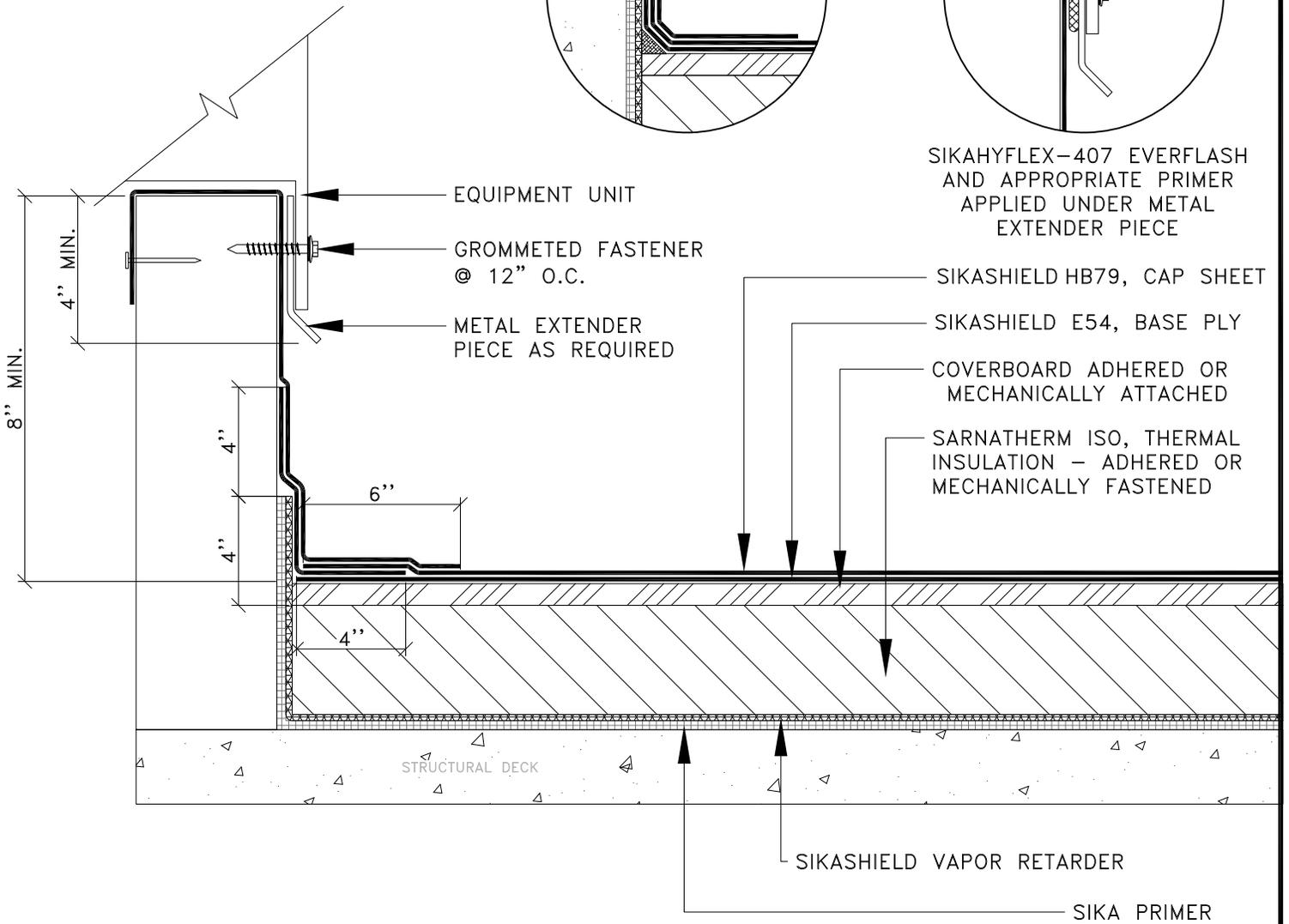
SIKAHYFLEX-407 EVERFLASH AND APPROPRIATE PRIMER APPLIED UNDER METAL EXTENDER PIECE
