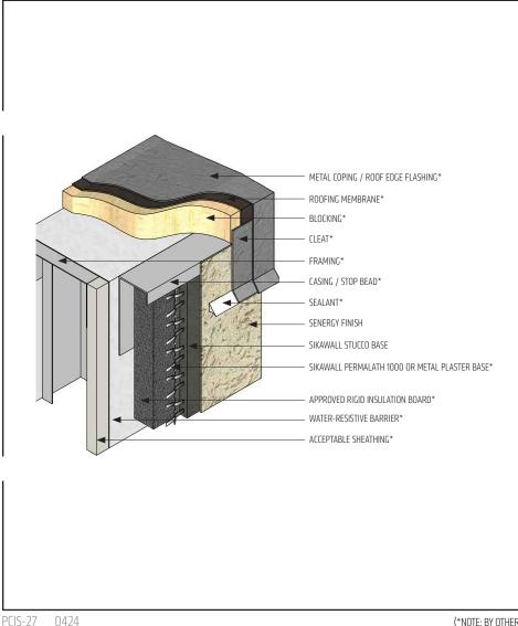
• It is recommended to lap coping or roof edge flashing over the Platinum CI Stucco system a minimum of 2" (50 mm) with drip edge sealed.
