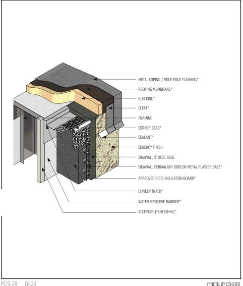
• It is recommended to lap coping or roof edge flashing over the Platinum CI Stucco system a minimum of 2" (50 mm) with drip edge sealed.
