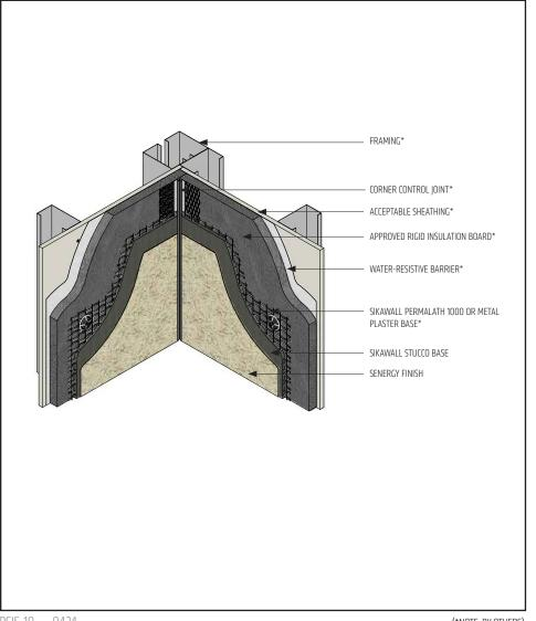
• Ensure water-resistive barrier application is continuous behind the Platinum CI Stucco system.
