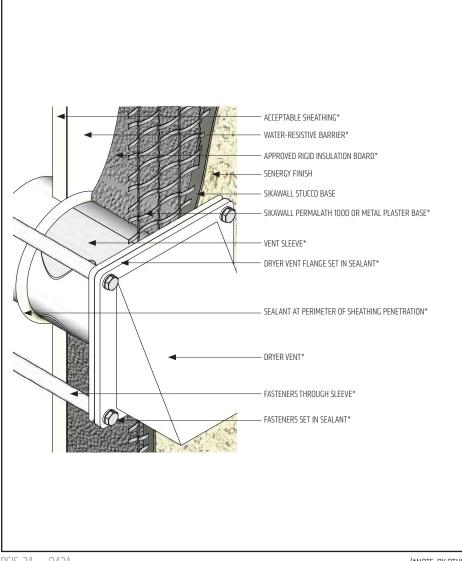
• Ensure all fastener penetrations through the Platinum CI Stucco system are properly sealed.
