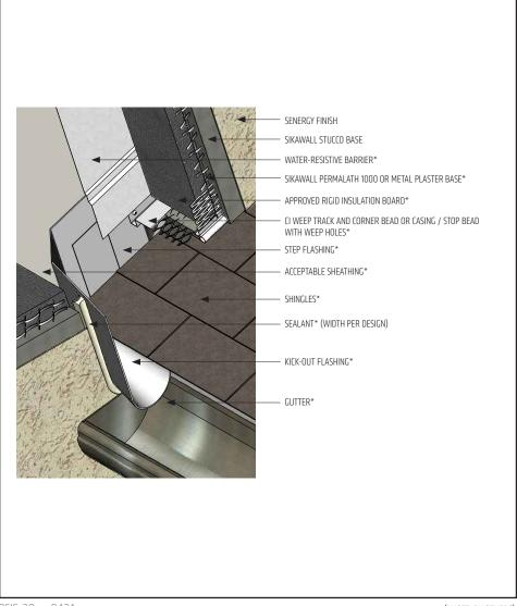
· Ensure water-resistive barrier laps over the CI Weep Track flange.
