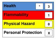
Caution: HMIS® rating is based on a 0-4 rating scale, with 0 representing minimal hazards or risks, and 4 representing significant hazards or risks. Although HMIS® rating is not required on SDSs under 29 CFR 1910.1200, the preparer may choose to provide them. HMIS® rating is to be used with a fully implemented HMIS® program. HMIS® is a registered mark of the National Paint & Coatings Association (NPCA). Please note HMIS® attempts to convey full health warning information to all employees.
