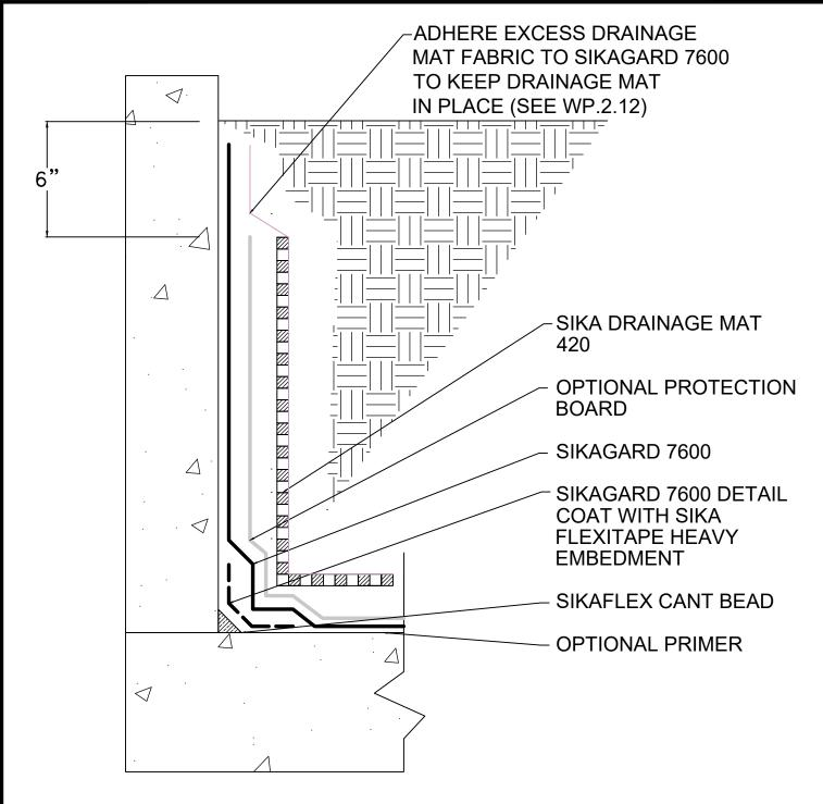
NOTES: REFER TO SYSTEM GUIDE FOR PRIMING, SIKAGARD 7600 THICKNESS, PROTECTION BOARD, AND DRAINAGE MAT
