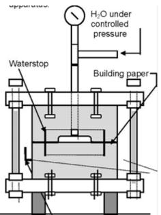
Based on test results for fluid migration, the U.S. Army Corps of Engineers recommends use of the conservative guidelines below for waterstop size selection.
