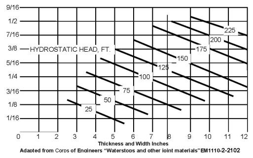
Additional factors must be considered beyond fluid migration when selecting a waterstop. These factors include the thickness of the concrete, location of reinforcement and mix design. Follow the parameters shown below.
