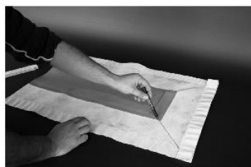
Position the trimmed tape section and mark on the bottom tape.
