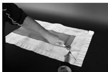
Position the cut tape and finish welding the sealing strip to the left and right.
