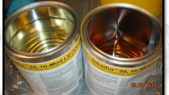
Mix thoroughly for 3 minutes with Jiffy mixing paddle on low-speed (400-600 rpm) drill until uniform in color
