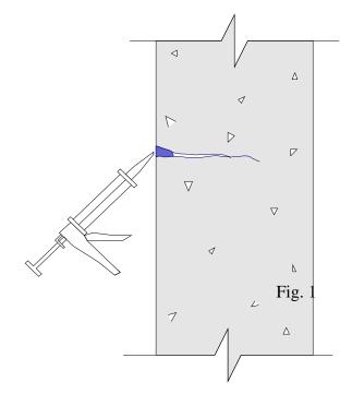
Figure 2 - Notch & Seal
