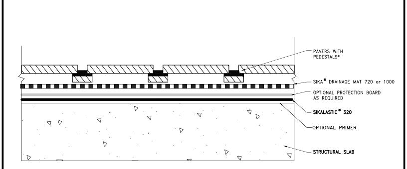
NOTES: REFER TO SYSTEM GUIDE FOR PRIMING, SIKALASTIC 320 THICKNESS, PROTECTION BOARD, AND DRAINAGE MAT REQUIREMENTS
