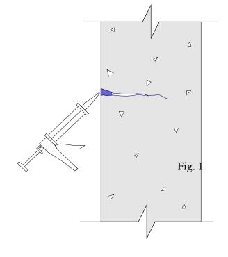
Figure 2 - Notch & Seal
