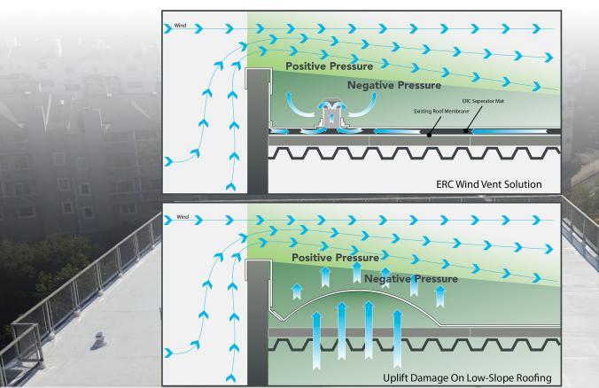
Uplift occurring on a roof is best explained by the Bernoulli's Principle. Bernoulli's principle states that an increase in the speed of a fluid occurs simultaneously with a decrease in static pressure or a decrease in the fluid's potential energy. In regards to roofing, the kinetic energy of the wind increases above a roof at the expense of pressure. For non-wind vent roofing system the negative pressure would lead to damage or even the tear off of a roof system.
