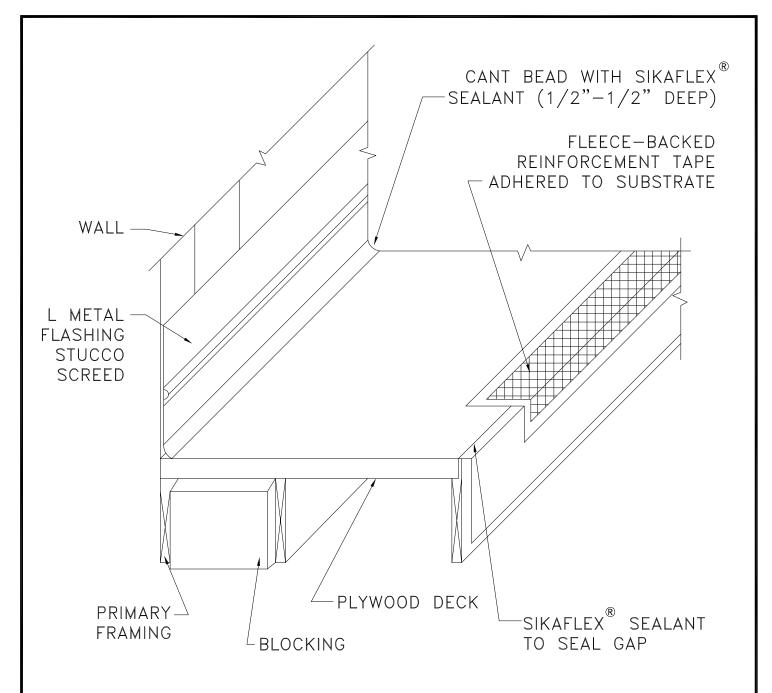
$\underline{\text{NOTE:}}$  SIKALASTIC  $^{\circledR}$  MEMBRANE NOT SHOWN FOR CLARITY. MEMBRANE TO BE INSTALLED ON PLYWOOD DECK, UNDER METAL FLASHING, AND TURNED UP WALL.
