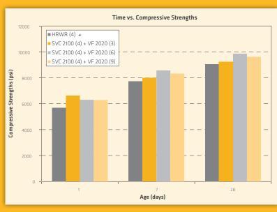
\*SVC 2100 - High range water reducing admixture • VF 2020 - Workability Retaining admixture • Dosage mentioned in bracket ( ) is fl. oz / 100 lbs. of Cm
