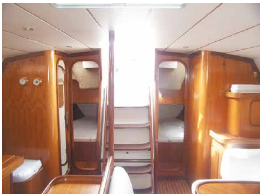
Fig. 90 High-quality lightweight panels finished in traditional high-gloss wood veneer and bonded using Sikaflex®-292
