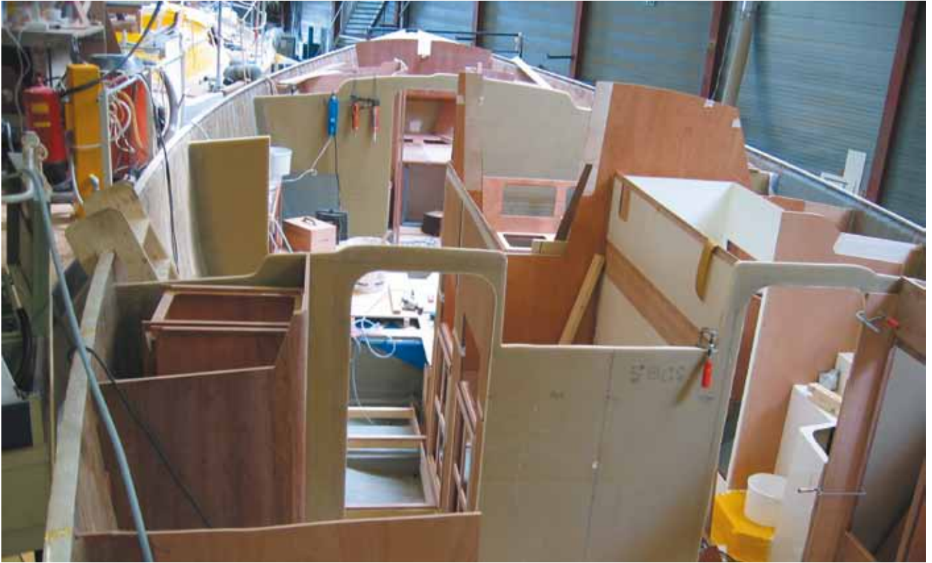
Fig. 91 Lightweight panels being fitted to an open hull
