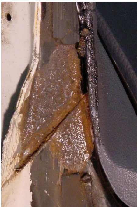
(Level 2 – 3 corrosion of pinchweld)
