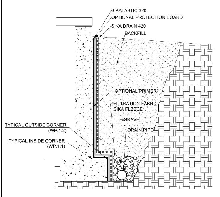
NOTES: REFER TO SYSTEM GUIDE FOR PRIMING, SIKALASTIC 320 THICKNESS, PROTECTION BOARD, AND DRAINAGE MAT REQUIREMENTS
